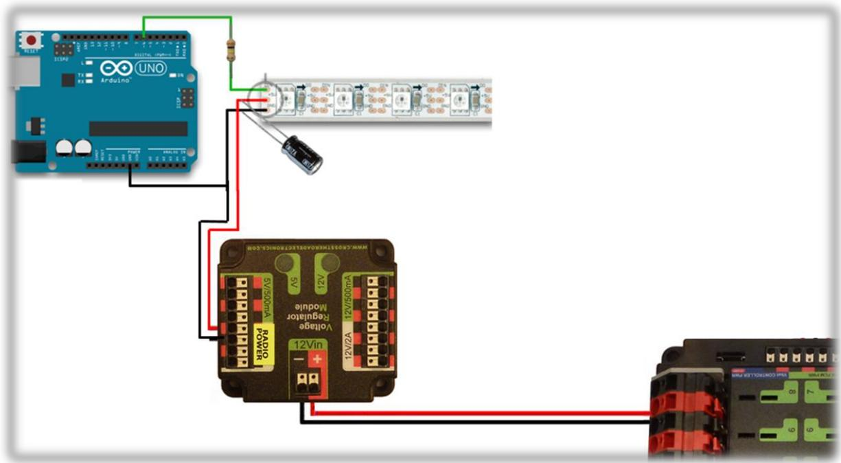
**Don't forget the 1000uF Capacitor and 300-500 Ohm Resistor!**
