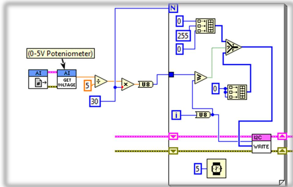
In this program (running in a larger loop), the output voltage of the 5V potentiometer is scaled to reflect an integer value between 0 and 30 (the number of LEDs in this test strip). In each iteration of the For Loop, this scaled value is compared with the iteration number. If the scaled value is *larger* than the iteration number, then the upper array is sent (corresponding to Green). Otherwise, the lower array is sent (corresponding to Off, or 0 0 0).
