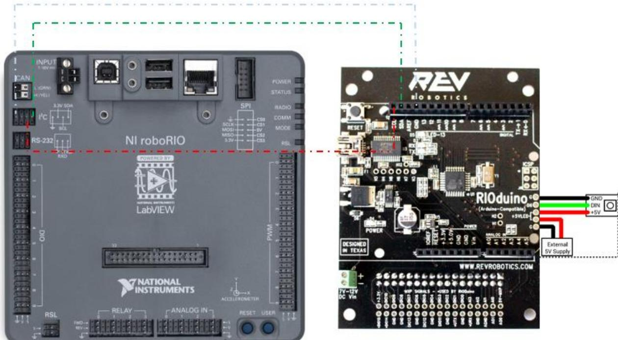
**Again, Don't forget the 1000uF Capacitor and 300-500 Ohm Resistor (Not Shown Above)!**
