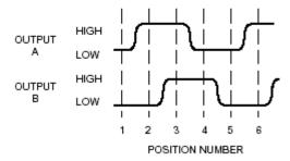
This diagram shows two important things. The first is the binary pattern of bits for phases (or outputs) A and B in each of the four positions.
