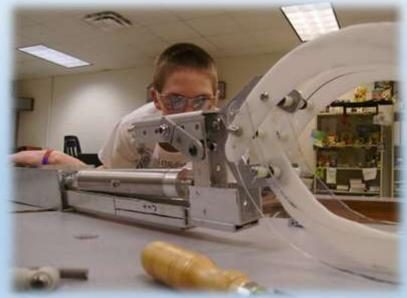
For every automated action/motion, a feedback sensor is required
