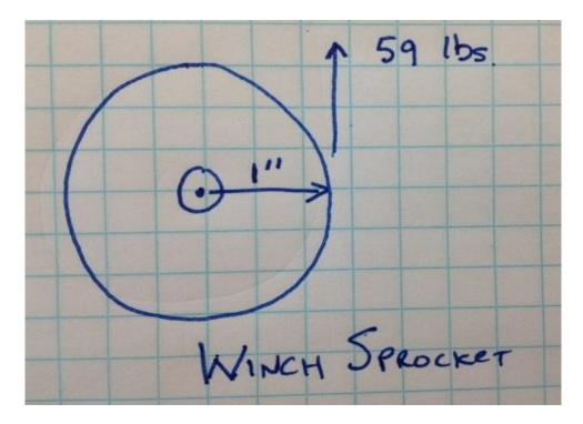
Speed and torque are inversely proportional (speed goes up, torque goes down). The torque at the gearbox output is 59 in-lbs so the torque at the gearbox input will be 59 in-lbs / 40 = 1.475 in-lbs. (The speed reduction through the gearbox is 40:1, so the input speed is 40 times higher than the output speed and the input torque is 40 times lower that the output torque.)
