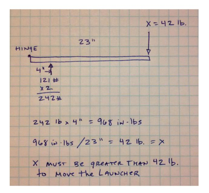
Before we determine the work required, we need to take another design factor into consideration. If we could pull the launcher straight down, it would take 42 pounds of force. But we will mount our winch near the back of the robot, so we will be pulling at an angle. This means that the vertical component of our pulling force must be 42 pounds, but the actual force from the winch must be higher than that.
