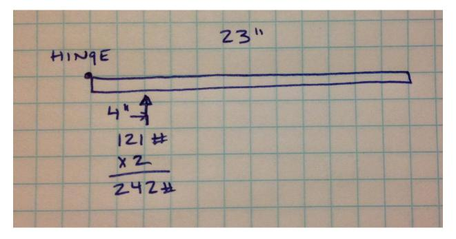
The springs we are using provide 121 pounds of force each and they are placed at 4 inches from the center of the hinge. To calculate the moment (torque), we multiply the Force times the Distance. There are two springs, so the Force is  $(2 \times 121)$  lbs = 242 lbs. Multiplying by 4 inches gives 968 in-lbs. The torque we need to overcome is 968 in-lbs.
