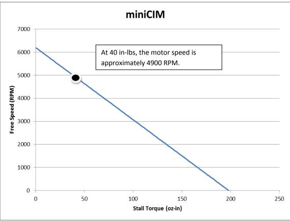
At 40 oz-in output torque, the CIM's output speed is ~4700 RPM. At 40 oz-in output torque, the miniCIM's output speed is ~4900 RPM. Since each of these speed points is higher than the speed where we need that torque output, both motors meet the requirement.
