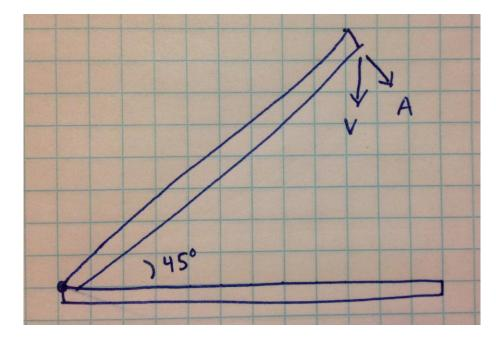
As noted in the sketch above, the launcher is at an angle after launching the ball and that angle point is the starting point for the pull. When the launcher is "up", it is at an angle of approximately 45 degrees. We will call the vertical component of this force V, and it is 42 pounds. We will be pulling at an angle, and this force is designated by A.
