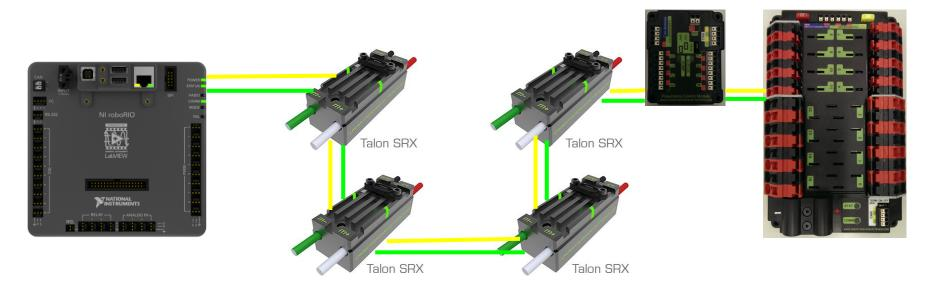
CAN (Controller Area Network) is a daisy chained communications bus where the two ends of the chain have a special terminator (see: <a href="http://en.wikipedia.org/wiki/CAN\_bus">http://en.wikipedia.org/wiki/CAN\_bus</a>).
