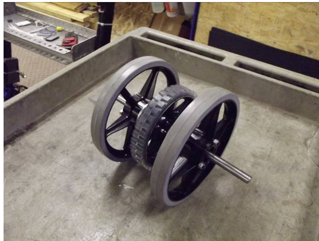
Pi's shooter. The center wheel was changed to non-treaded later.
