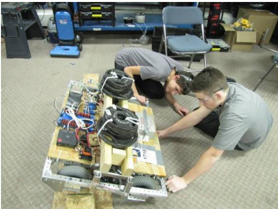
The kitbot at full weight with pneumatic wheels and front lead-ins. Too bad it didn't turn well.
