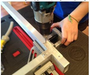
g. Frequent check with machine square and check diagonal distance with measuring tape to ensure everything is square.
