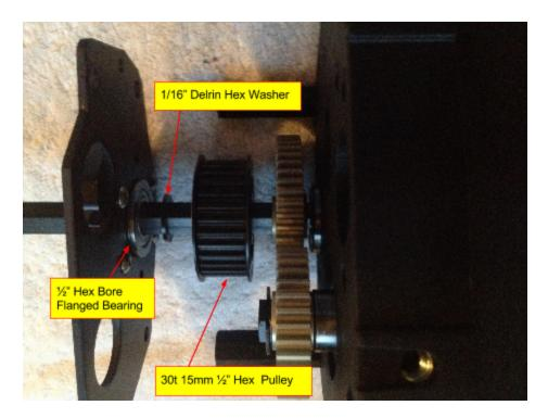
e. You also need a 1/16" delrin hex washer between the pulley and the flange bearing of the WCD 3rd stage plate.
