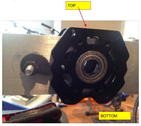
c. Some bearing need to be pressed in with a one ton press and some you need a retaining compound like loctite 680 to keep it in place
