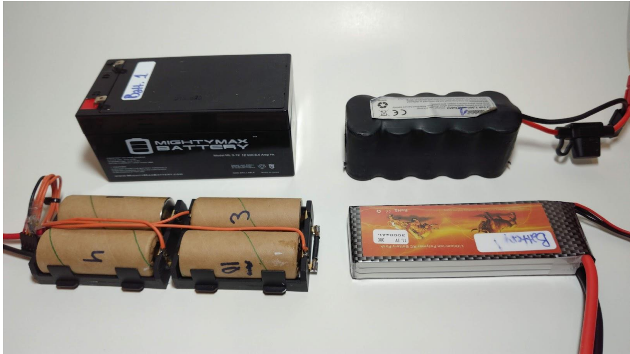
Figure 4: The battery chemistries used for testing. Top Left: Lead Acid, Top Right: NiMH, Bottom Left: LiFePO 4 , Bottom Right: LiPo
