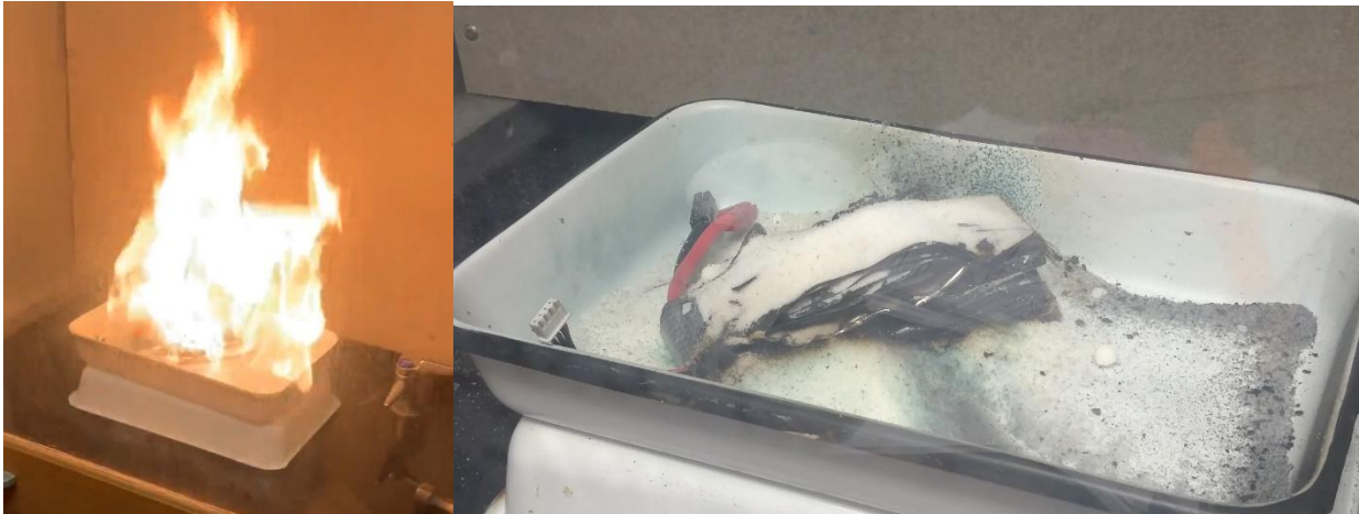
Figure 12: Lithium Polymer battery during and after nail-intrusion test.
