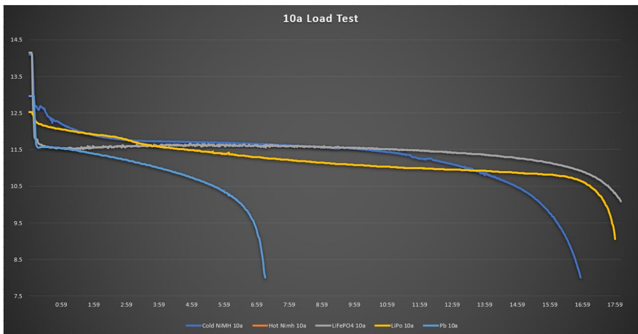
Figure 9: A graph of discharge curves at a current of 10 amps
