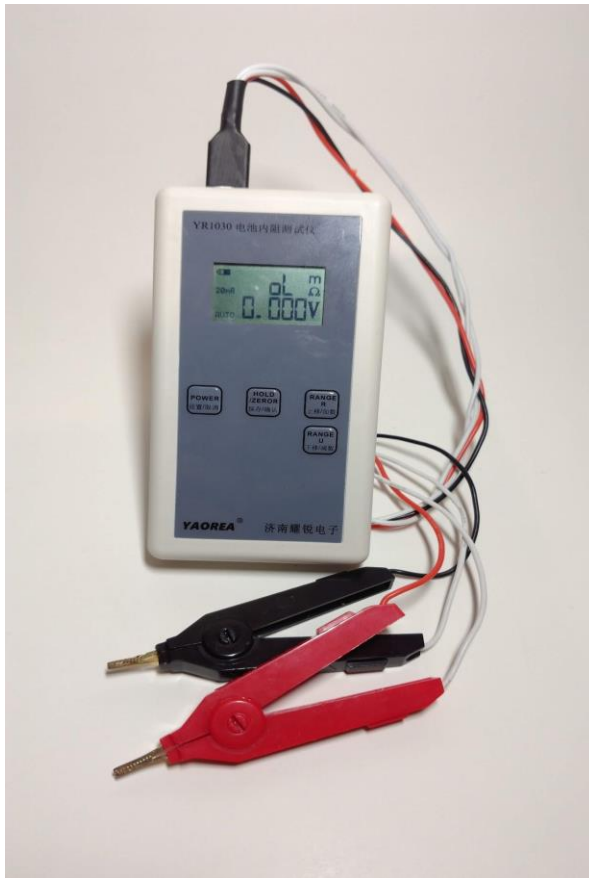
Figure 6: YR1030 Internal Resistance meter; uses AC Conductance to measure internal resistance.
