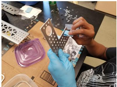
2. Once the part is clean, cut a length of wire and make it into an 'S' (or tall 'C') shape. Hang the wire on the rack and hang the part on the wire.
