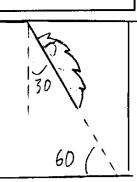
BEVEL vs. MITER: A miter refers to an angle cut across the flat surface of a board. Miters are generally cut with a chopsaw or with a tablesaw, using a MITER FENCE to make a crosscut.
