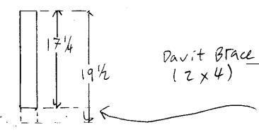
Option E: (Static disk) If not making lower disk, make davit bracket longer so disk is still at correct height.
