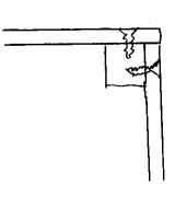
Glue blocks need to have two absolutely smooth sides at a particular angle. Start with a scrap piece of 2 x 4 and rip two edges at the approriate angle to make an approximately 1 1/2 x 1 1/2 strip with two adjacent freshly-cut sides. (Drill appropiate clearance holes, usually 5/32 for #8 screws.)
