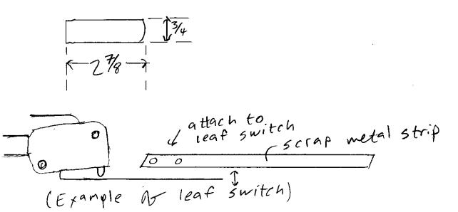
Attach the switches to the lower davit brackets so they are actuated by the disk dowel when the lower disk is elevated.
