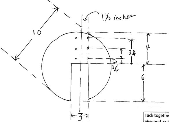
Tack together 6 layers of 3/4 plywood, cut out circle and notch on bandsaw.
