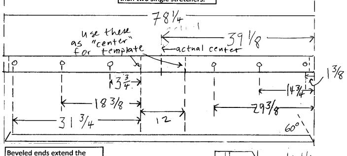
Beveled ends extend the beveled edges of the Outer Supports. Length at the end (past the hole to connect to the Outer Support) is slightly shorter than for the Single Base Stretcher, since its Outer Support is single beveled.
