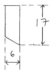
When the lower plates are laminated with the upper plates, they are not centered, since one end forms part of a 1 1/2 inch groove and the other end forms part of a 3 inch groove.
