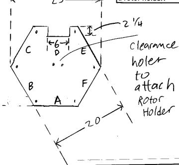
Slightly undersized - 23 inches corner-to-corner to fit inside steam tank skin and make 24 inch corner-to-corner steam tank.
