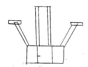
The steam tank is built up from pillars which fit into notches in hexagonal plates. The steam tank can be removed from the airship.
