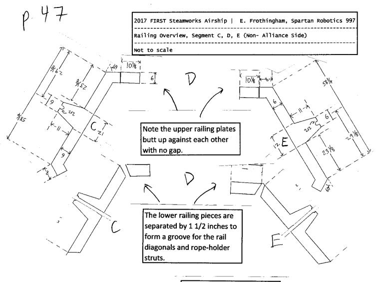
If the grooves do not come out right, they can be widened with a router, or narrowed by attaching glue blocks on either side of the groove.
