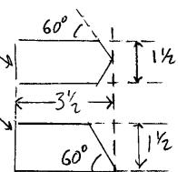
Forms corners of airship deck, connects to base stretcher and is glued and screwed to rail diagonal.
