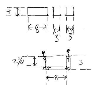
Cut and screw as shown to make 2 1/4 by 8 space to hold gear.
