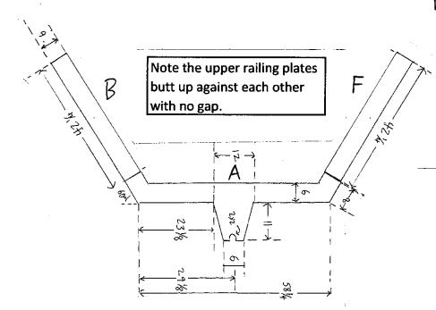
Note that the lower rail plates on the alliance side extend out to articulate with the extended upper rail plates on the non-alliance side.
