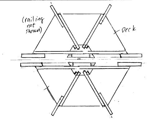
Rope lifts (davits) jut out from the center of the railing in three segments; the rope lifts are supported by diagonal struts.
