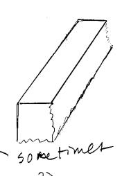
Quick bulletproof joint: Apply glue to block. Use template to drill clearance / pilot holes 3/4 inch from edge of vertical sheet, screw block to vertical sheet. Apply glue to seam and top of block, use nailer to tack horizontal board in place, then use template to drill pilot/clearance holes 1 1/2 inch from edge. Screw to block.
