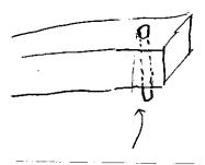
What if I goof? Make some "goof plugs" - start with 5/16 dowels. Trim them down a little for 9/32 inch holes (I used a block plane), cut to 2 1/2 inch lengths and taper one end slightly with a pencil sharpener. If you drill a hole wrong, hammer in a glued "goof plug", then cut off the ends and re-drill.
