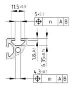
The ø 4.3 mm core bore for M5 is reborable up to max. ø 6 mm or M6.
