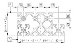
Modular dimension/position and dimensional and positional tolerances of grooves and core bores as a function of the profile's exterior dimension.
