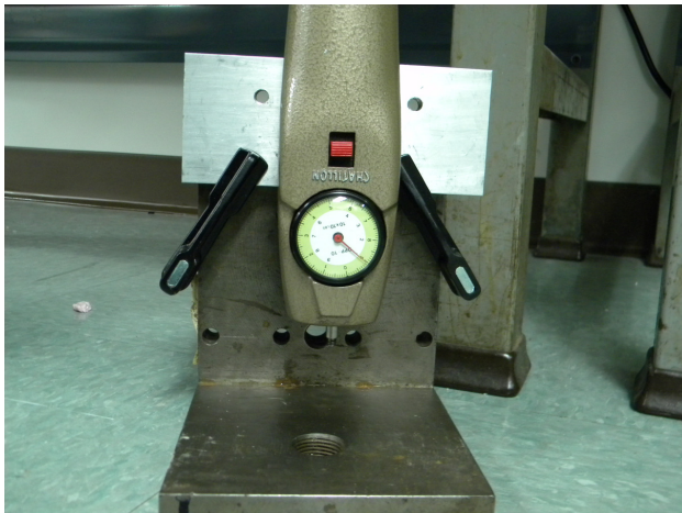
Figure 6 Force gauge indicating 1 lb tension with DC source.
