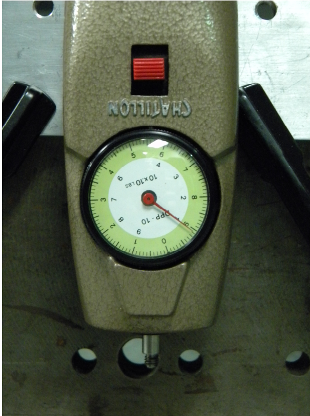
Figure 9 Tension when powered by Talon SRX at ~6 Amps.
