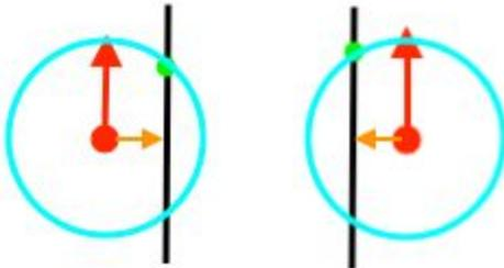
In these cases the distance to the lookahead point is the same, but in one the robot needs to turn right and in the other, left. We need to know what *side* the lookahead point is on. If we imagine the robot as a vector (red) and robot-to-lookahead-point as a vector (orange), we can take the sign of the cross product of the vectors to calculate if the lookahead point is on the left or right. If the answer is positive, the point is on the right, if it is negative, left.
