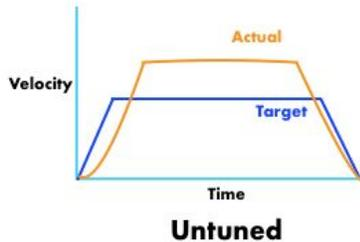
$K_v$ : Pick a  $K_v$  approximately equal to  $1/(\text{top robot speed})$ . With the other constants set to 0, run the path. Adjust  $K_v$  until the target and measured velocities match up when the robot is traveling a constant speed.
