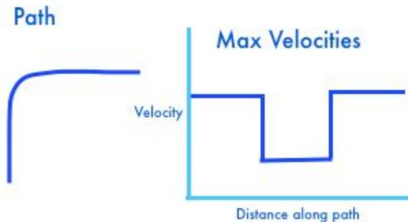
As the path curves more the target velocity decreases. And even though  $1/\text{curvature}$  may approach  $\infty$  at points, the velocity is constrained by the path's max velocity.
