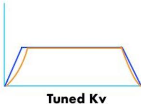
$K_a$ : Start  $K_a$  around 0.002. Adjust until the target and measured velocities match decently (don't worry about perfection) when accelerating, cruising, and decelerating.
