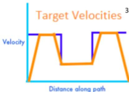
This produces a problem. The robot's target velocity is based on which point it is closest to, and in this graph the point at the start of the path has a velocity of 0. The robot would never start to move. To fix this, we remove the smooth acceleration and leave only the deceleration:
