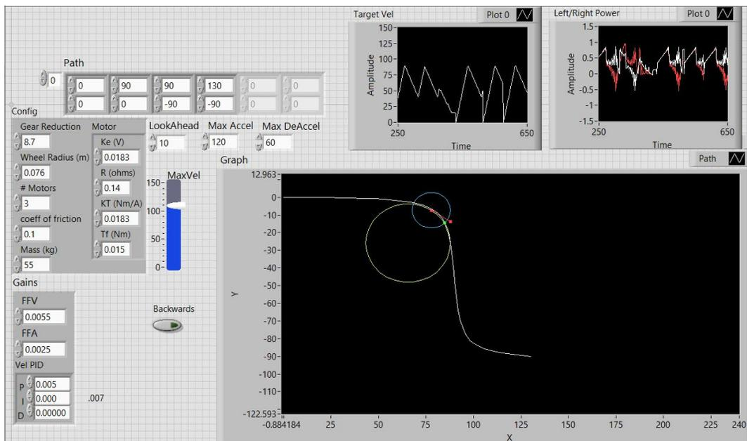
We simulated a robot by simulating two motors (one for each side of the drive) then using skid-steer kinematics to calculate what the robot's sensors would be reading. You can do a google search for these topics if you want to try implementing a robot simulator.
