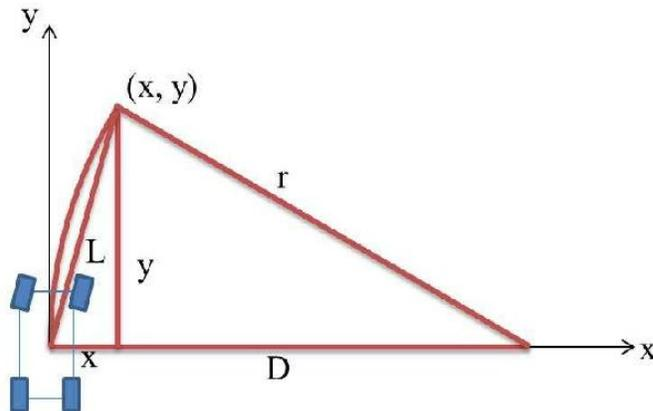
In the above diagram, the X and Y axes are aligned with the robot. L is the lookahead distance, (x, y) is the lookahead point, r is the radius of the arc, and D is simply the difference between r and x . From basic math we have:
