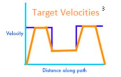
This produces a problem. The robot's target velocity is based on which point it is closest to, and in this graph the point at the start of the path has a velocity of 0. The robot would never start to move. To fix this, we remove the smooth acceleration and leave only the deceleration:
