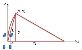
In the above diagram, the X and Y axes are aligned with the robot. L is the lookahead distance, (x, y) is the lookahead point, r is the radius of the arc, and D is simply the difference between r and x. From basic math we have:
