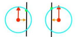
In these cases the distance to the lookahead point is the same, but in one the robot needs to turn right and in the other, left. We need to know what *side* the lookahead point is on. If we imagine the robot as a vector (red) and robot-to-lookahead-point as a vector (orange), we can take the sign of the cross product of the vectors to calculate if the lookahead point is on the left or right. If the answer is positive, the point is on the right, if it is negative, left.
