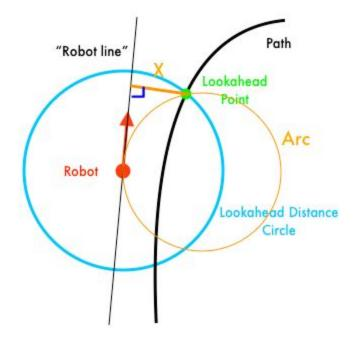
We use the point-slope formula to find the equation of the "robot line":
