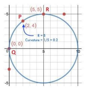
Derivation: (method 2 of <u>https://www.qc.edu.hk/math/Advanced%20Level/circle%20given%203%20points.htm</u>) Given three points P(x1, y1), Q(x2, y2), and R(x3, y3), we are trying to find the circle with center C(a, b) and radius r that intersects P, Q, and R. We can write r = |PC| = |QC| = |RC|. The solution to this is:
