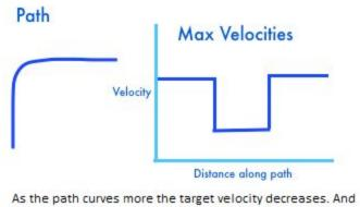
As the path curves more the target velocity decreases. And even though  $1/curvature may approach \infty$  at points, the velocity is constrained by the path's max velocity.
