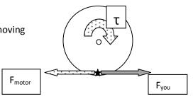
b) If the motor applies torque, the associated force on the edge of the wheel is pointing **in the plane of the wheel** (note: we are NOT looking at the force the <u>wheel</u> puts on the <u>ground</u>-THAT is the force for which mecanum will be at an angle. This is the force the motor is putting on this particular bit of the wheel)
