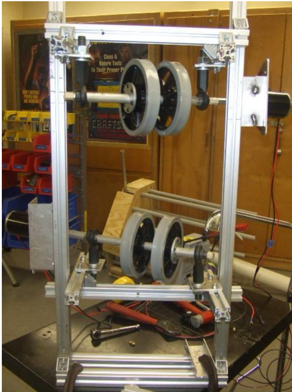
Figure 2 - Shooter Prototype with Direct Drive CIM's 1
