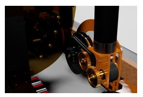
We chose this design over the tube-in-tube elevator design we saw a lot of teams build in 2020 due to its light weight and intuitive design. We believed that with a little bit of prototyping, and the resources found online for 118-style climbers and other steel-tape climbers, we could build an effective climber that was lighter, faster, and easier to build than the elevator climbers.
