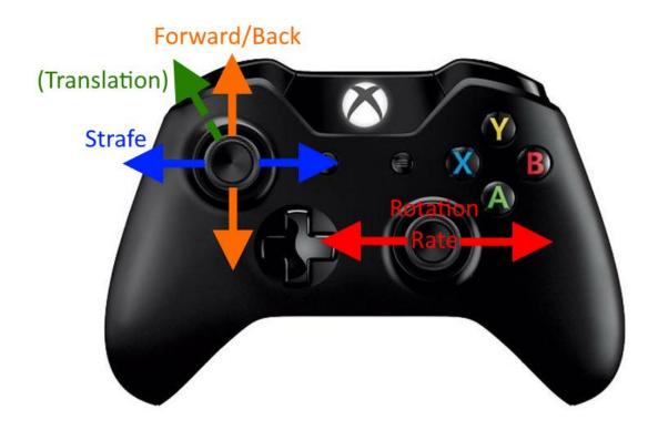
Each of those controls (orange, blue, and red) can be read in the robot program giving us an "analog" value from -1.0 to 1.0. The Forward/Back (orange axis) would be the X component of our translation vector (positive forward), and the Strafe (blue axis) would be the Y component (positive to the left).
