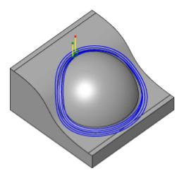
The **Pencil** strategy creates toolpaths along internal corners and fillets with small radii, removing material that no other tool can reach. Whether using single or multiple passes, the **Pencil** strategy is ideally suited for cleaning up after other finishing strategies.
