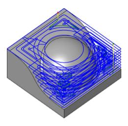
**Pocket** is the conventional roughing strategy for clearing large quantities of material effectively. The part is cleared layer by layer with smooth offset contours maintaining climb milling throughout the operation. To avoid plunging, the tool ramps down along a helical path between levels. To maintain a high feedrate, and thereby reducing machining time, sharp changes of direction are avoided by smoothing the tool motion.
