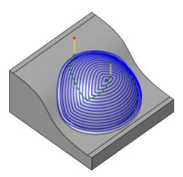
The **Scallop** strategy creates passes that are at a constant distance from one another by offsetting inward along the surface. The passes follow sloping and vertical walls to maintain the stepover. Although **Scallop** finishing can be used to finish an entire part, it is most commonly used for rest
