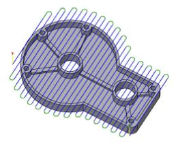
The **Facing** strategy is designed for quick part facing to prepare the raw stock for further machining. It can also be used for clearing flat areas in general.
