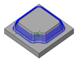
**Contour** passes is the best strategy for finishing steep walls, but can be used for semi-finish and finish machining on the more vertical areas of a part. If a slope angle is specified, for example 30 to 90 degrees, the steeper areas are machined, leaving the shallower areas up to 30 degrees for more appropriate strategies.
