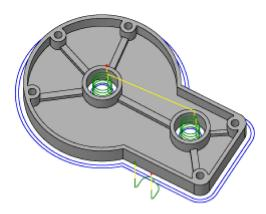
With the **Contouring** strategies, you can easily machine 2D and 3D contours with separate lead-in and lead-out, and with or without tool compensation. Choose multiple roughing and finishing passes and multiple depth cuts for any contour. Machine open and closed contours without creating additional geometry and eliminate sharp motion with corner smoothing.
