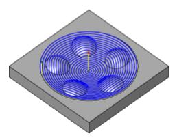
**Spiral** machining creates a spiral toolpath from a given center point, generating a constant contact as it machines within a given boundary. It is ideally suited for use on round shallow parts using tool contact angles up to 40 degrees, in conjunction with **Contour** passes for the more vertical faces. The center point of the detail to be machined is located automatically, or can be user-specified. This strategy also supports tool contact angles.
