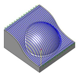
**Parallel** passes is one of the most widely used finishing strategies. The passes are parallel in the XY plane and follow the surface in the Z direction. **Parallel** passes are best suited for shallow areas and down milling. To automatically detect shallow areas, the machining can be limited to a maximum angle between the tool tip and the surface. By selecting the down milling option, tool deflection can be minimized when machining complex surfaces.
