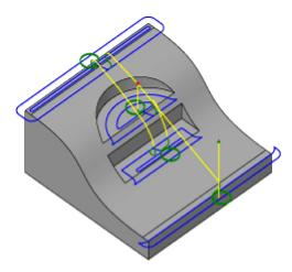
The **Horizontal Clearing** strategy automatically detects all the flat areas of the part and clears them with an offsetting path. When the flat area is shelved above the surrounding areas, the cutter moves beyond the flat areas to clean the edges. Using the optional maximum stepdown, horizontal faces can be machined in stages, making the horizontal clearing suitable for both semi-finishing and finishing.
