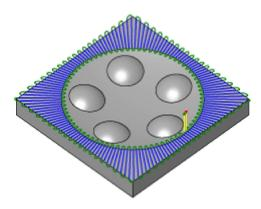
Like spiral machining, **Radial** machining also starts from a center point, providing you with the ability to machine radial parts. It also provides the option to stop short of the center of the radial passes, where they become very dense. The center point of the detail to be machined is located automatically, or can be user-specified. This routine can also be used with tool contact angles.
