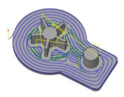
The **Adaptive Clearing** strategy creates a roughing/clearing toolpath inside closed curves both with and without islands. This strategy avoids full-width cuts by progressively shaving material off the remaining stock. The generated toolpath ensures that the cutting conditions remain constant with a stable load on the tool. As a result, the feedrate can be increased significantly, reducing the machining time by 40% or more which provides improved surface quality and less tool wear.
