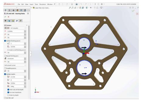
Set finishing passes to 0. Also set multiple depths with a max stepdown of .125 in. Also set Even Stepdowns and Finish Only At Final Depth. Select the plunge holes for the Predetermined positions.
