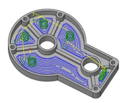
The **Pocket** toolpath is used for machining closed curves both with and without islands. The toolpath starts at the center of the pocket and works its way outward. The entry can be selected anywhere on the model and includes possibilities for plunge, ramp, or at a pre-drilled position. The special high-speed option creates a smooth toolpath and allows you to specify a maximum tool
