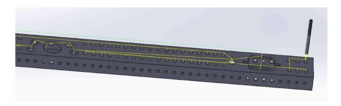
Use a ½" EM for the bearing block holes (this is the 3 flute, carbideEM, with a .0004in chip load at 5400 RPM) This is necessary to get the slots. Select the top contours of both bearing block holes and access holes. In the heights section set Bottom to from Stock Top to "-0.155". Then set multiple depths at .06 with even step downs. This will give 3 passes.
