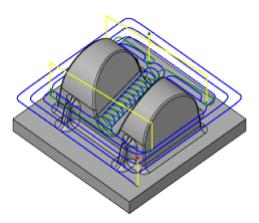
**Adaptive Clearing** is an innovative roughing strategy that offers significant improvements compared to conventional roughing strategies. The strategy avoids full-width cuts by progressively shaving material off the remaining stock. The generated toolpath ensures that the cutting conditions remain constant with a stable load on the tool. As a result, the feedrate can be increased significantly, reducing the machining time by 40% or more.
