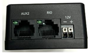
PoE + 12 VDC is the recommended method per R617 Using passive PoE cables is compliant with R703 B This is the recommended method for redundant power
