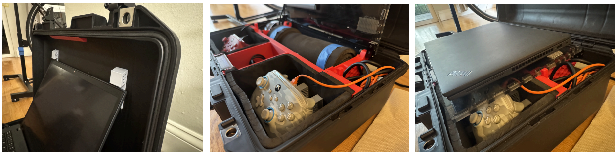
(Left) Laptop lid tabs to hold the case lid open when the laptop is open. (Center, Right) Controller pocket inserts that hold the controllers up to avoid resting on and straining the USB connector.
