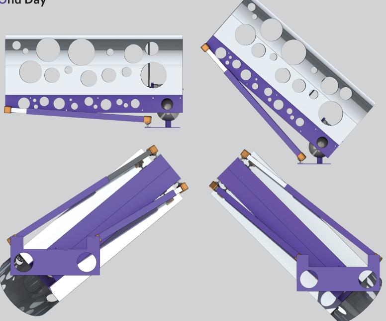
The manipulator is mounted on a 4" □al-tec™ Kinematic Element, and is actuated by a pair of ball-screw linear actuators. The large 2-dof range of motion allows for precise and flexible alignment during the match.
