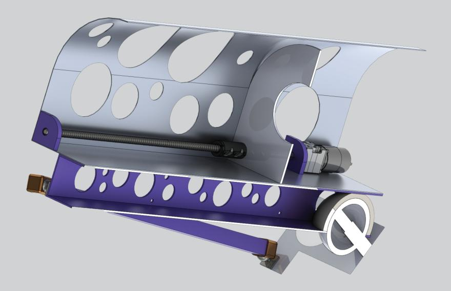
The intake receives balls from the human player station. To score, the ball-screw driven paddle pushes the spheres back out.
