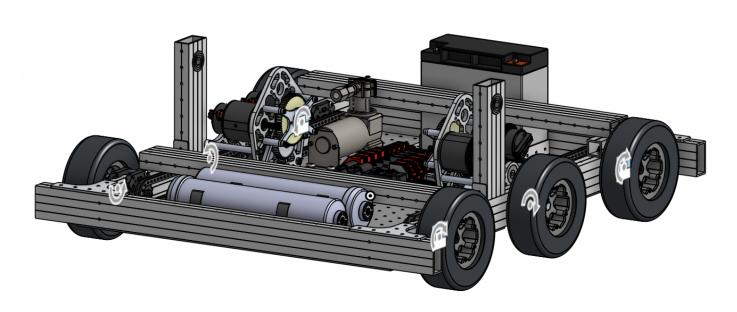
Our drivebase was very similar to the one fielded in the 2020 competition. It is designed to be simple to assemble, manoeuvrable, and have high acceleration rather than top speed.
