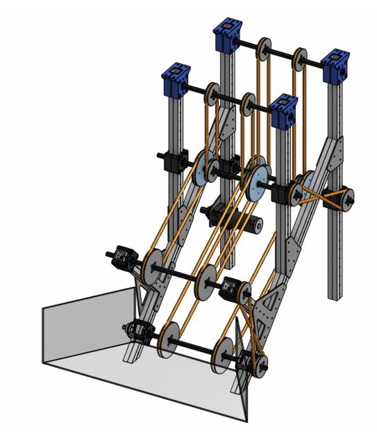
The indexer is designed to carry balls from the intake to the shooter reliably. The size of the indexer was designed to allow the shooter to shoot balls over a climber design we had in mind. It also had to provide a constant speed to the balls entering the shooter to ensure consistent shots. We intended to do this without a 'kicker' like in our 2020 robot to enable a simpler design.
