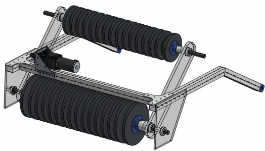
The intake was heavily inspired by the #118 Robonauts design. Given we started building our robot later in the year we decided to copy many elements of it. It particularly stuck out because of its interesting foam rollers and 'over the bumper' design.
