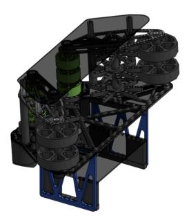
The indexer complements the intake by reorienting the coral in the proper direction for the rest of our Coral path. And allows us to intake Coral faster.
