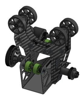
The Scoring mech allows us to hold and score Coral as well as take algae off the reef. This one mechanism controls both game pieces and works with our other intake mechanisms
