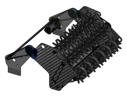
The intake allows us to pick up Coral from the ground at any orientation. This allows us to be more competitive and run fast cycles that don't necessarily depend on human coral input.
